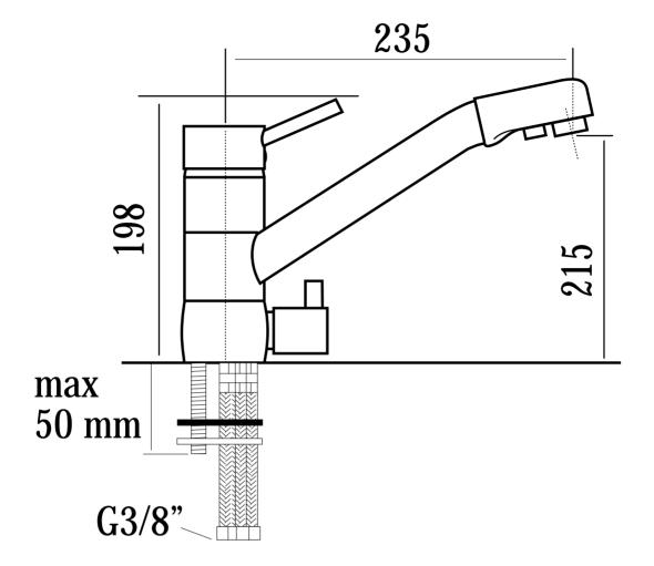
maximum sink hole diameter 32-35mm diametro massimo foro lavello 32-35mm
