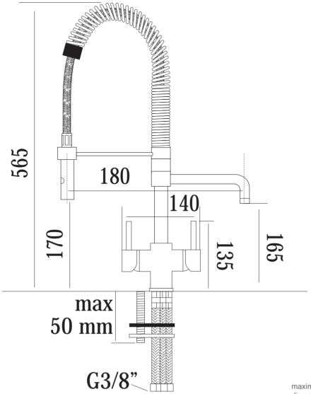
maximum sink hole diameter 32-35mm diametro massimo foro lavello 32-35mm
