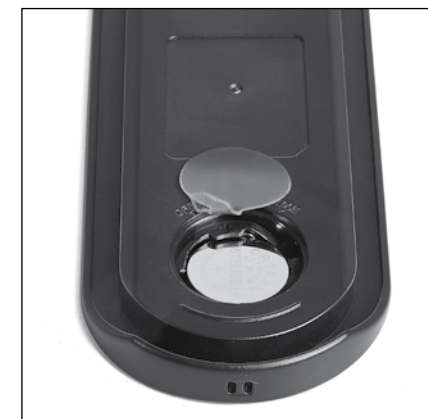
Fig. 2 Remove the plastic tab and replace the battery correctly.
