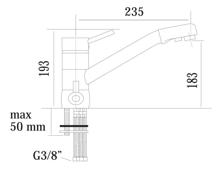
maximum sink hole diameter 32-35mm diametro massimo foro lavello 32-35mm
