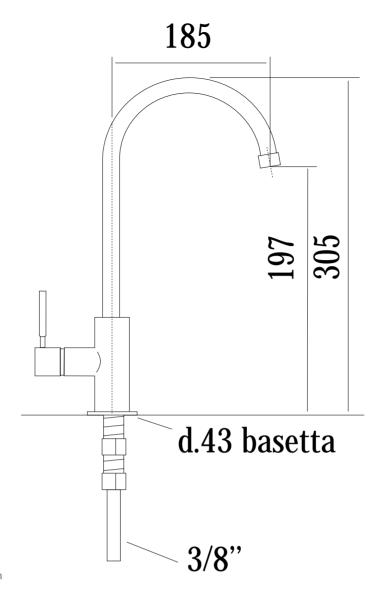
maximum sink hole diameter 32-35mm diametro massimo foro lavello 32-35mm
