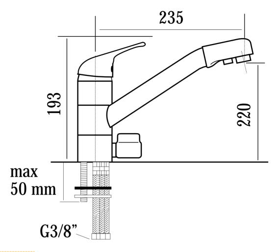
maximum sink hole diameter 32-35mm diametro massimo foro lavello 32-35mm
